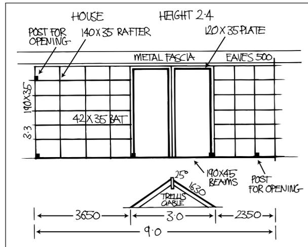
before you start. Mark and prepare your site with stakes and level string lines as per your floor plan, measuring along your string line to mark the location of your upright posts. Double check all your measurements and ensure everything's square by measuring diagonally. Dig all post holes to specified size. Remember the string line is at the outer edge of all external posts.
